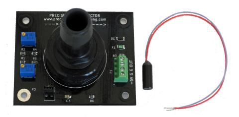
Galvanometer scanners need encoders for accuracy. Polygon scanners require Start-Of-Scan detection for accuracy. This SOS kit is plug and play. It will give the most accurate results from any polygon scanner. It zeros out facet to facet error. (Don't use an encoder on a polygon scanner. An encoder introduces runout error and cannot accurately tell you where the scan starts or where the beam is pointing!)
